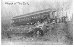
junction. Then it was attached to the rear coach, and pulled the train into New Boston by moving backwards. With the engine running backwards, that put the tender (carrying the coal) in the front of the entire train. On the afternoon of March 27, 1909, the train was running in this manner, when the tender
